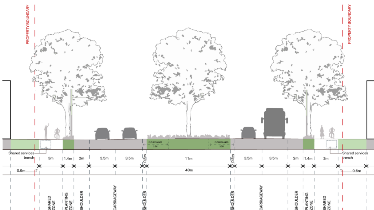
Figure 5.3 Appin Road and East-West Connection Road typical cross-section
